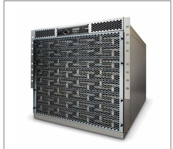
SeaMicro SM10000 high density, low power server.
